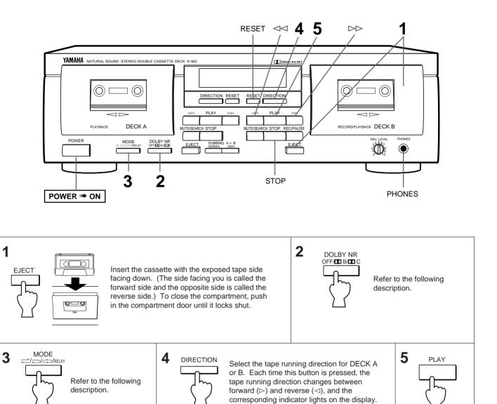
To fast forward or rewind the tape When the tape running indicator  $\triangleright$  is lit: Pressing the  $\triangleright \triangleright$  button fast forwards the tape while pressing the  $\triangleleft \lhd$  button rewinds the tape. When the tape running indicator  $\lhd$  is lit: Pressing the  $\triangleleft \lhd$  button fast forwards the tape while pressing the  $\triangleright \triangleright$  button rewinds the tape.
